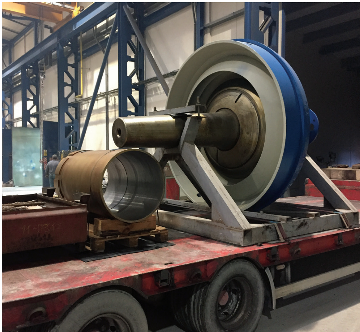
Supporting cone repair – SY 1067 (cone diameter 2 200 mm)
