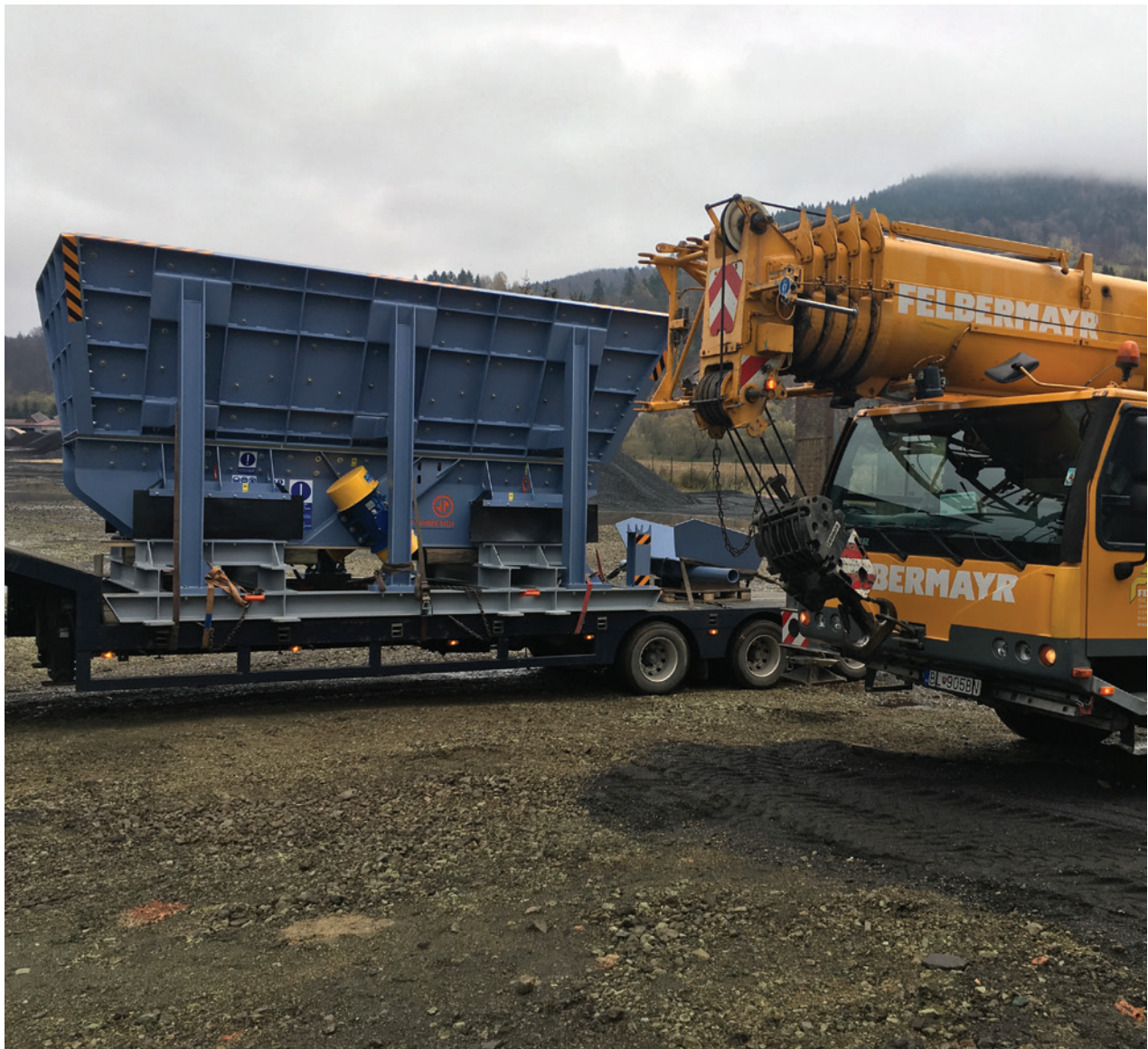
Vibrating feeder VPF 1050, including receiving hopper 15 m³
